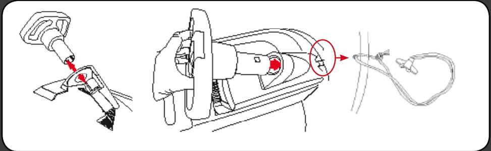
GB Mounting/ Slide the steering wheel into the tube until it is completely fastened.
