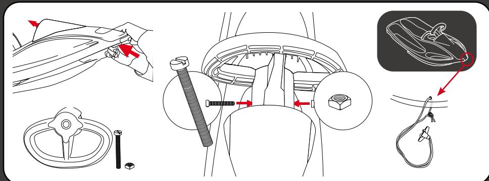
GB Slide the steering wheel over the metal tube and fasten with the screw and nut. Fasten the pulling rope.
