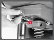
To take the seat off, press the release button (1b) up and hold. Now rotate the rear of the seat upwards (a) and then pull it (b) rearwards.
